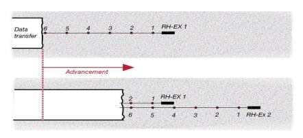
*Figure 2.18 shows the application of the Reverse Head Extensometer in Alptransit Gotthard tunnel Switzerland.*
