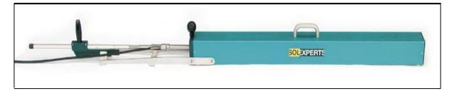
Figure 2.9 shows the complete set of calibration devices of Sliding Drformeter.
