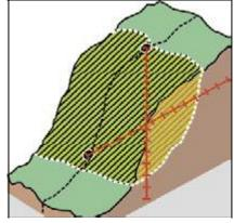
Monitoring of strain development and displacement along boreholes in soil and soft rock as well as it is to measure displacements in swelling rock during tunnelling and monitoring of the tunnel portals and portal slope, figure 2.7.
