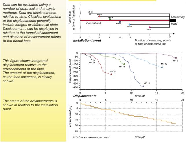
Figure 2.19 shows the application of the Reverse Head Extensometer at Alptransit Gotthard base tunnel Switzerland.
