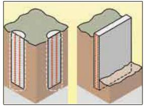
It is for Geotechnical Strain Profile Measurements. The Sliding Deformeter is a development of the Swiss Federal Institute of Technology, Zurich (ETHZ). Sliding Deformeter is for deformation measurements in Geotechnical applications in soil and soft rock.
