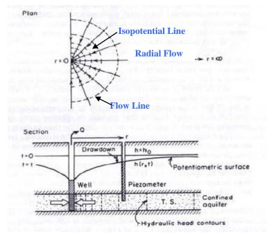
Figure 3.1 shows single well, interference test (Cross hole test).
