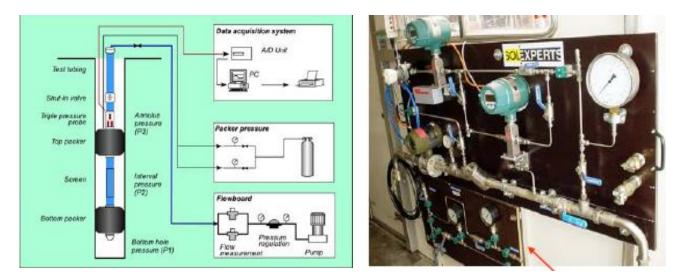
*Figure 3.5 shows double packer test equipment arrangement for testing after borehole is completed.*
