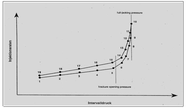
Figure 2.49 Flow rate plotted versus injection pressure of hydrojacking test.
