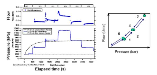
Figure 3.3 shows some examples of water pressure test (Lugeon test) results.
