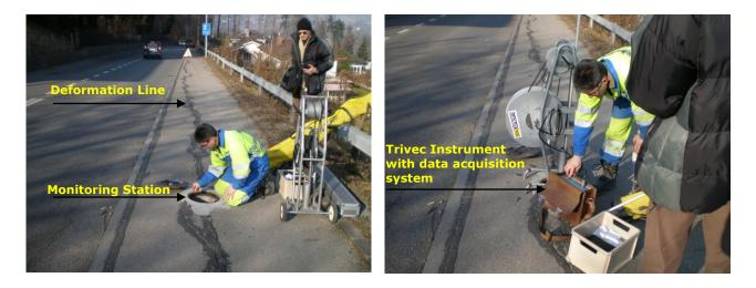
Figure 6.14 shows the measurement of slope movement X, Y and Z vector by Trivec probe on road side slope at Maur.
