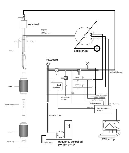
*Figure 2.50 schematic overview of a hydrojacking double packer layout of the test system and the surface equipment.*
