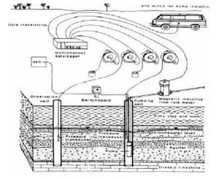
Figure 3.2 shows the complete field set up of the pump test.
