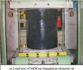
protection sleeve  $\emptyset$ =900 mm, and H=1000 mm
