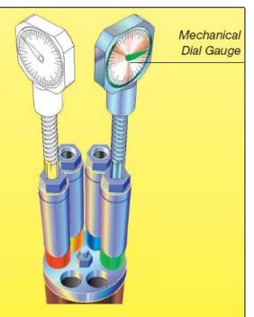
For the manual measurement of the multi-point Extensometers, a dial gauge or the portable electronic displacement transducer with digital readout unit is used.
