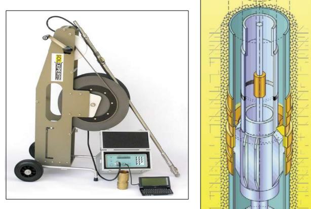
Figure 2.10 shows complete set of Sliding micrometer and internal details of the probe.
