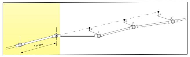
Figure 2.32 shows the function of chain deflectometer in a multiple automatic monitoring of subsurface deformation.
