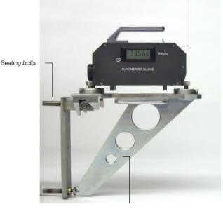
Figure 2.28 shows the instrument set up and use Clinimeter BL200B.
