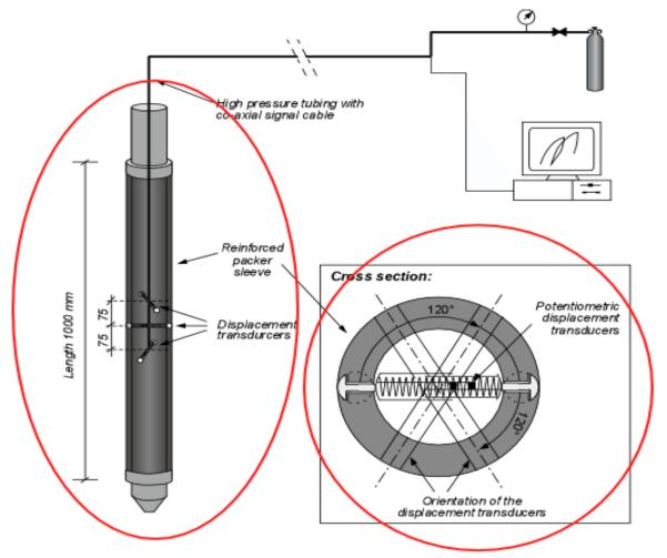
Figure 2.34 shows the internal structural details of the dilatometer probe
