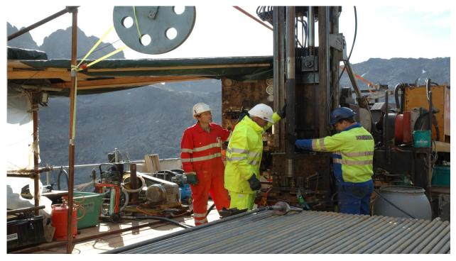
Figure 2.35 Installation of the dilatometer probe in exploratory borehole for Emosson pumped storage hydropower plant (Switzerland) Dilatometer probe, Sedimentation tube and Installation rods.
