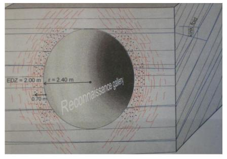
Figure 6.12 Shown a model of excavation disturbed zone (EDZ).
