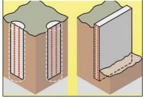
Figure 2.13 shows the use of sliding micrometer at piles and diaphragm walls.
