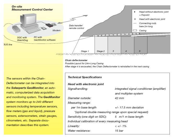
Figure 2.33 shows the application of chain deflectometer on pipe canopy at tunnel crown.
