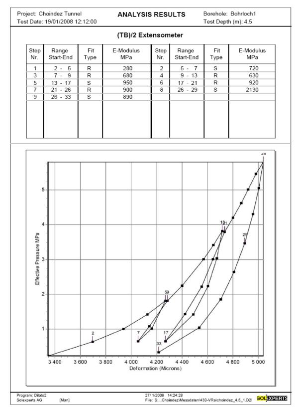
The above presented chart and data is an example of the dilatometer test result at the depth of 4.5m.
