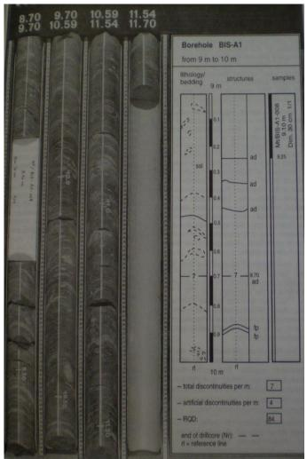
*Figure 6.11 shows the careful handling and systematic arrangement of the drill core before logging.*
