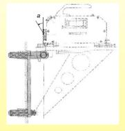
Seating bolts VB, for measuring change in inclination in the vertical plane parallel to the wall.
