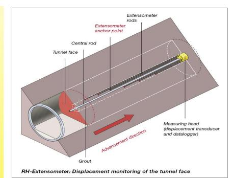
Readout of the frequently saved data is made at the tunnel face.
