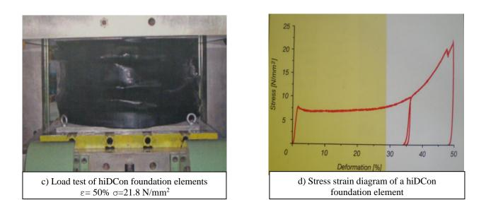
Figure 5.2 a, b, c, and d shows test result of deformability constant resistance for application in squeezing and swelling rock soil in tunnels.
