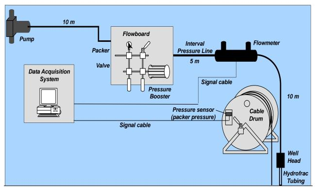
Figure 2.45 showing the arrangement of the surface equipment arrangement.
