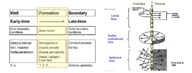
Figure 3.7 shows the flow regimes and flow model in Double Packer test.
