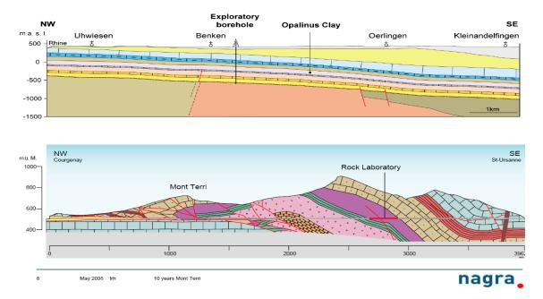
Figure 6.9 a simplified NW-SE geological profile through the Mont Terri anticline.
