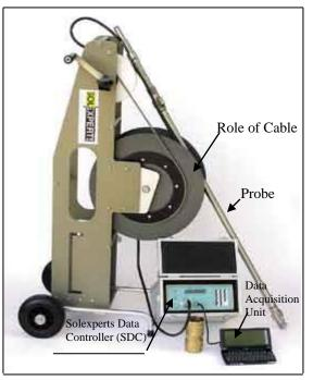
Figure 2.1 TRIVEC measuring equipment.
