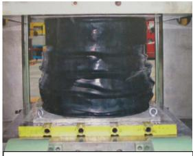
b) Load test of hiDCon foundation elements  $\epsilon{=}~25\%~\sigma{=}7.4~N/mm^2$
