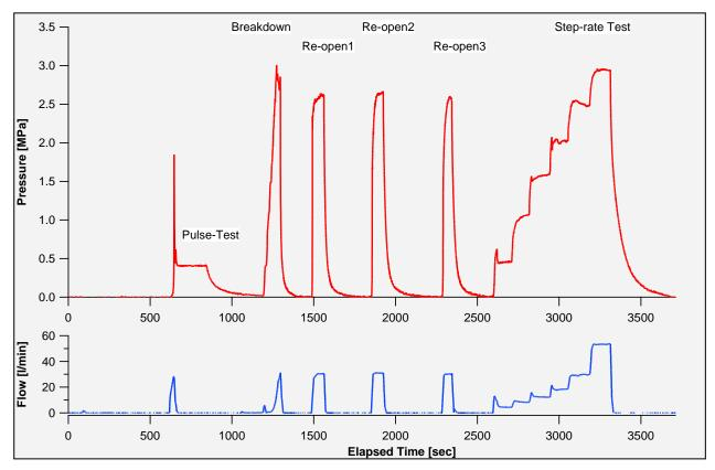
Figure 2.46 shows the results of hydraulic-fracturing test with breakdown cycle, the re-open cycles and a step-rate test.
