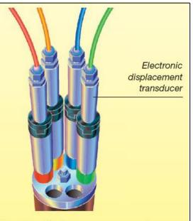
For automatic distance measurements ofthe Extensometers, electronic displacement transducers are installed.
