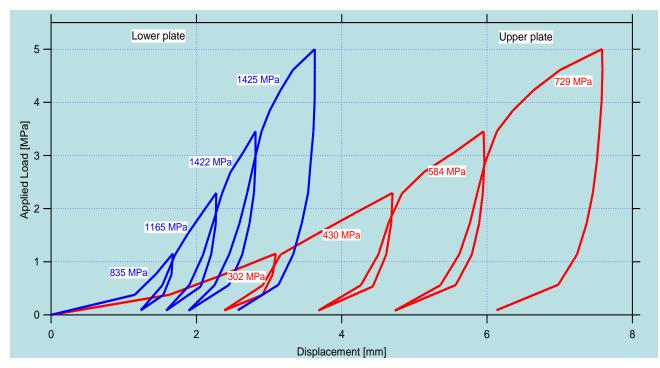
Figure 2.41 an example of plate loading test results with four cycles and corresponding value of the deformation module. A stiffening of the rock mass with increasing rock load is observed with both plates.
