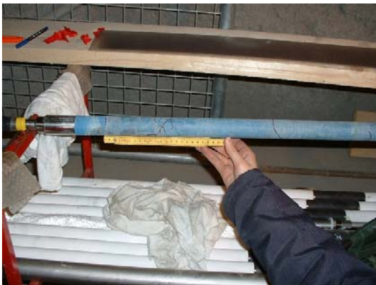
Figure 7. Original fracture traces on impression packer
